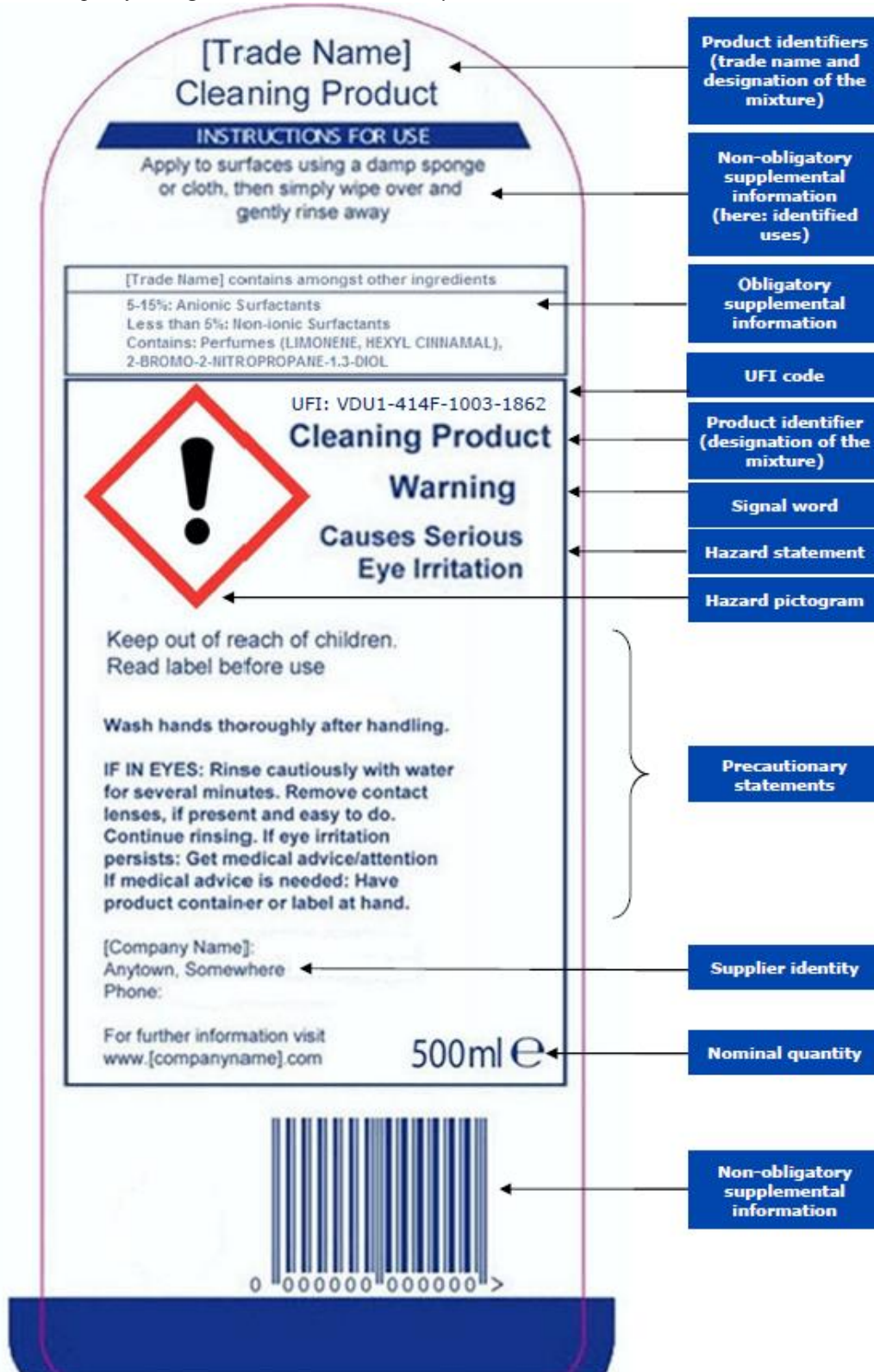
Figure 90: Example of detergent label. Hazard class "Eye Irritation" 89
